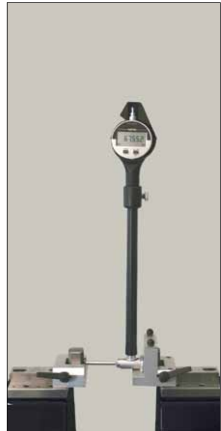
Setting of 2-point bore gauges (TEL5/TA-SU-301)
