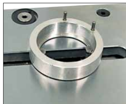
Checking of internal grooves (TELS10)
