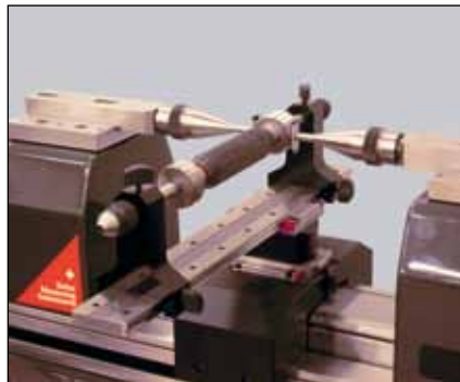
Checking of thread plug gauges (HPA-1/TEL6/3P/0.17-3.2/S6.5/LABC-15)
