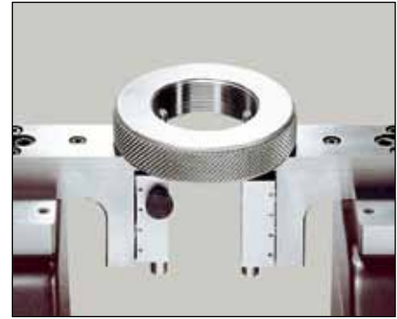
HPA: Checking of thread ring gauges (TEL18)
