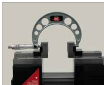
Checking of external micrometers (TEL5/TEL11)
