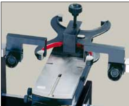
Checking of snap gauges (TA-SU-313/TEL14N)
