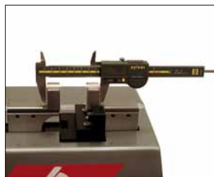
Checking of calipers
