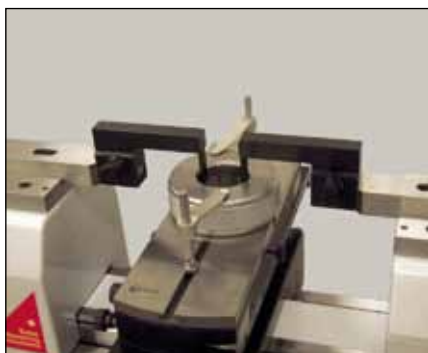
Etalonnage de bagues lisses (TA-SU-313/TEL16.1/HPA-1)
